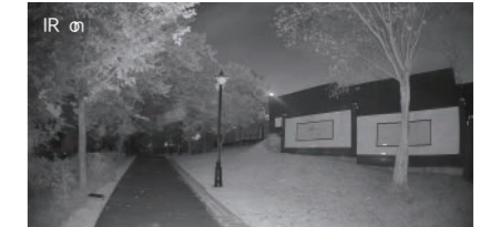
Camera switches back to IR mode automatically after targets leaving the monitoring area, white light LED is off, IR LED is on.
