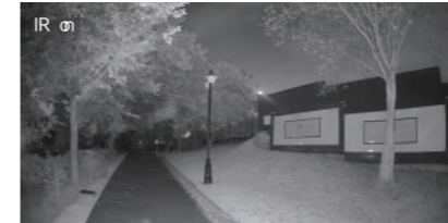
Camera stays in IR mode with no target (human / vehicle / non-motor vehicle) entering into the monitoring area, IR LED is on, white light LED is off.
